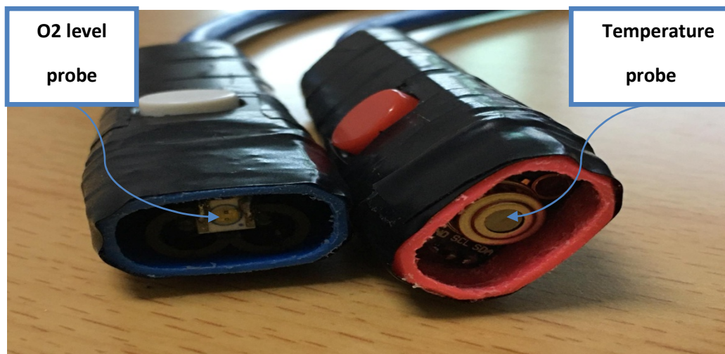
Figure 6.1 Probes of the temperatures and O 2 sensors
