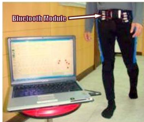
Figure 3.23. Wireless gait analysis system by digital textile sensors.
