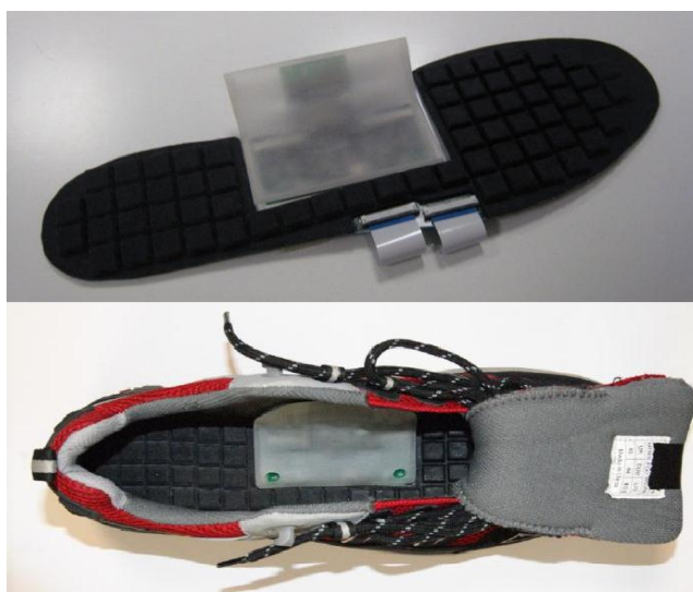
Figure 3.35. De Rossi et al. insole sensor system and the system fitted inside a shoe.
