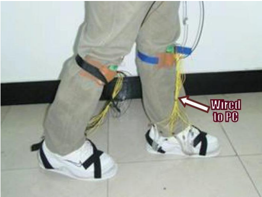
Figure 3.16. Identification based on dynamic plantar pressure in-shoe system
