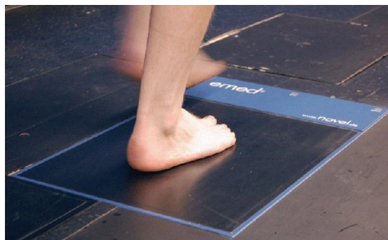
Figure 3.1. A platform-based foot plantar pressure sensor (static)
