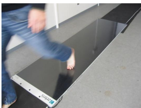
Figure 3.2. A platform based foot plantar pressure sensor (dynamic)
