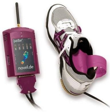
Figure 3.3. An in-shoe based foot plantar pressure sensor (uniform)
