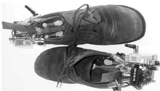
Figure 3.21. Shoe-integrated wireless sensor system, Gait Shoe, showing all the hardware components.
