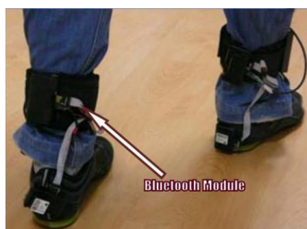
Figure 3.22. A wireless system for gait and posture analysis based on pressure insoles and inertial measurement units.
