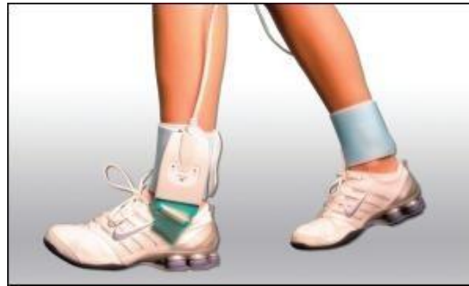
Figure 3.4. An in-shoe based foot plantar pressure sensor
