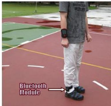
Figure 3.25. In-shoe plantar pressure measurement and analysis system based on fabric pressure sensing array
