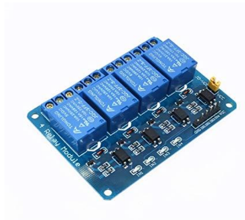
Figure 3.8: 4 Channel relay switches module.
