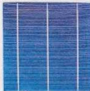
Figure 2-9 Multicrystalline PV cell
