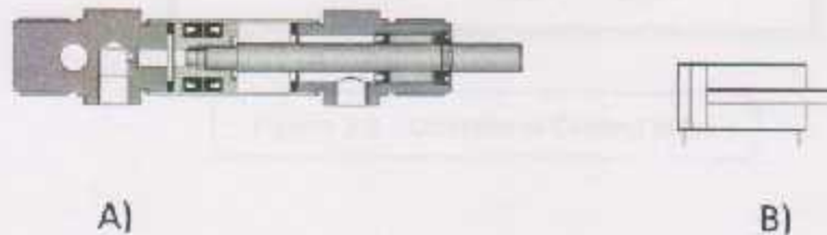
Figure 3.7: The Cylinder Type A) Double Acting Cylinder B) symbol Of Double Acting Cylinder
