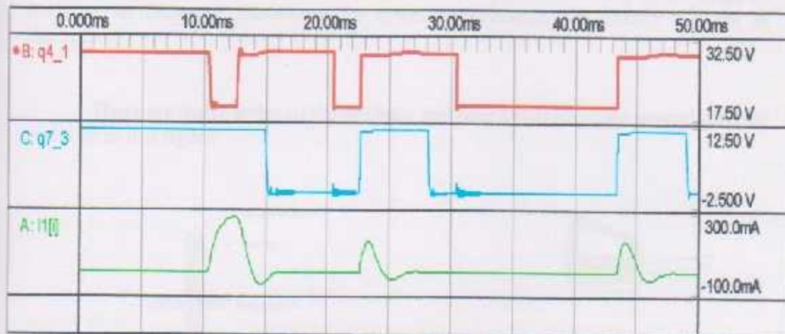
Fig 9.13 : Output waveform for defibrillator .
