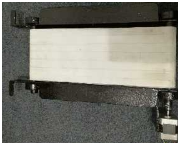
Figure 5.1: conveyer with stepper motor
