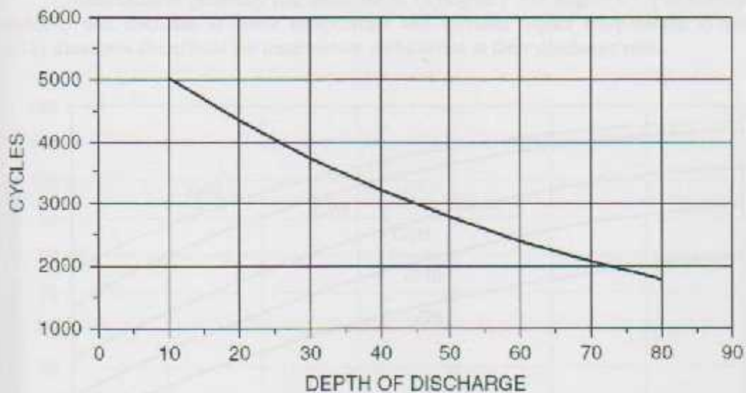
Figure 2.10: Impact of Depth of Discharge on the Number of Cycles [10]
