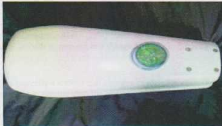
Figure 4.4: Photocell Mounted At the Top of Street Lighting Fixture [45]
