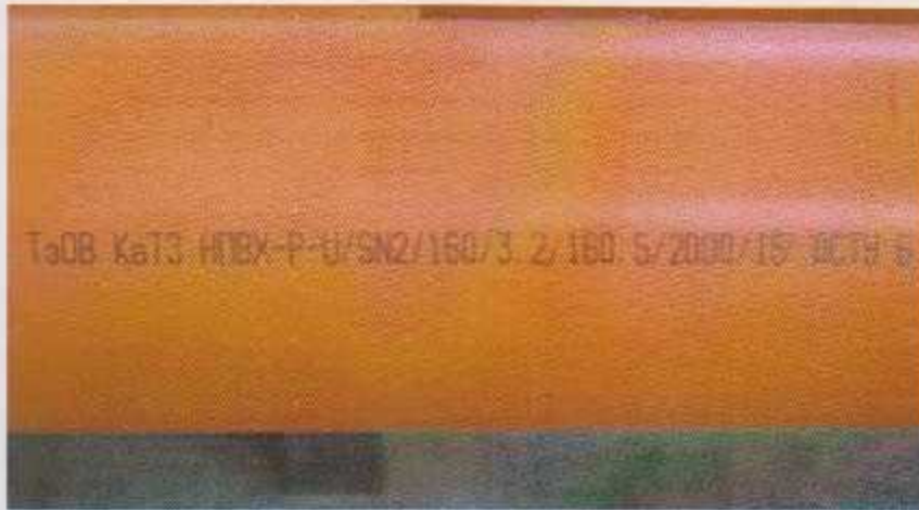
Figure (2.2): Plastic pipe made from PVC material.
