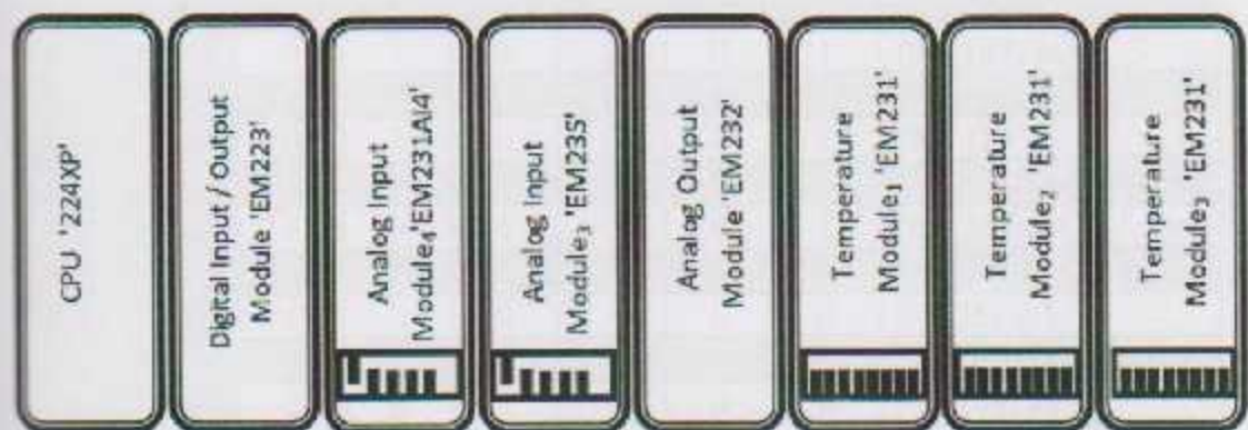
Figure (6.3): Hardware configuration of PLC.
