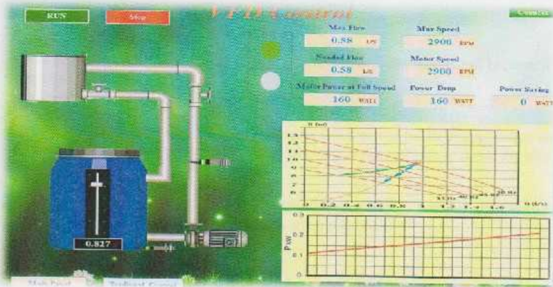
Figure 5.18 VFD Monitoring Screen
