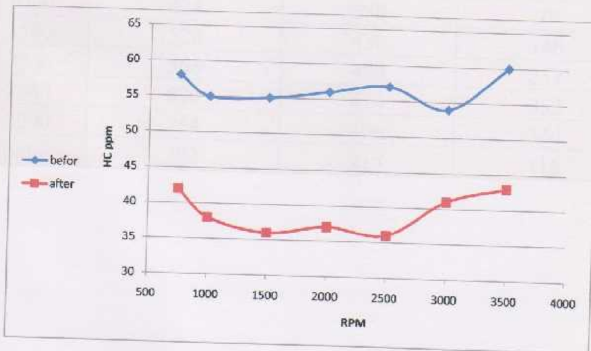
Figure (6.6): HC emission versus engine speed (before and after catalytic converter)
