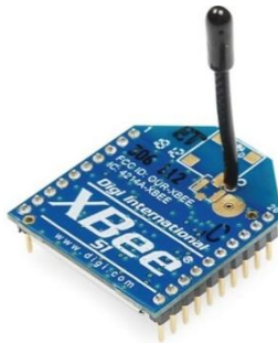
Figure 3.7: The XBee 1mW wire antenna- series 1
