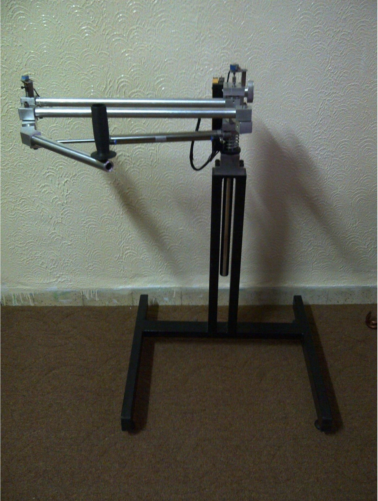
Figure 9.4: The mechanical structure with the load system, the three sensors and the control box
