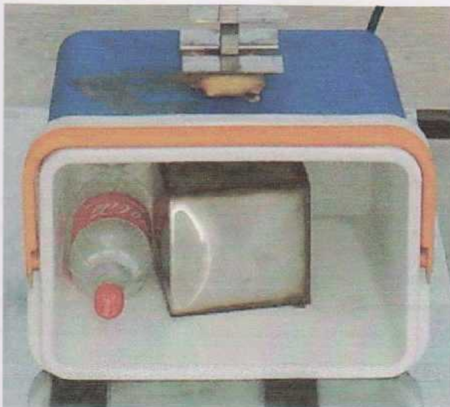
Figure 2.7 ice box and receiver tank
