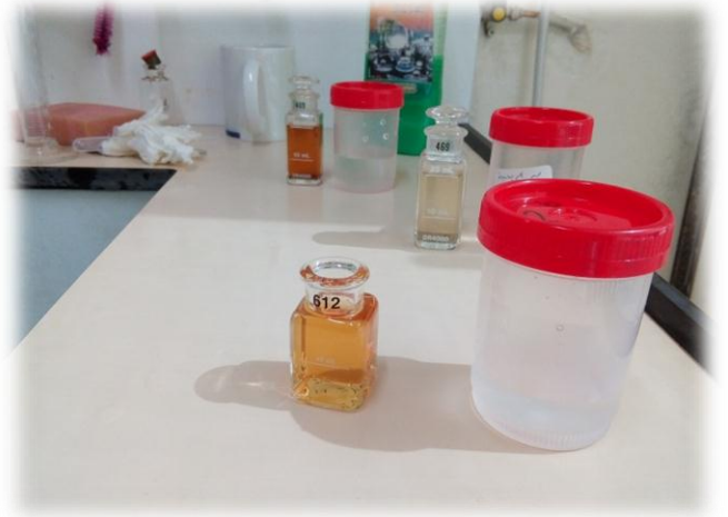
Figure 6.9: the red colored of the wells samples after adding the powder to measure the absorbance.
