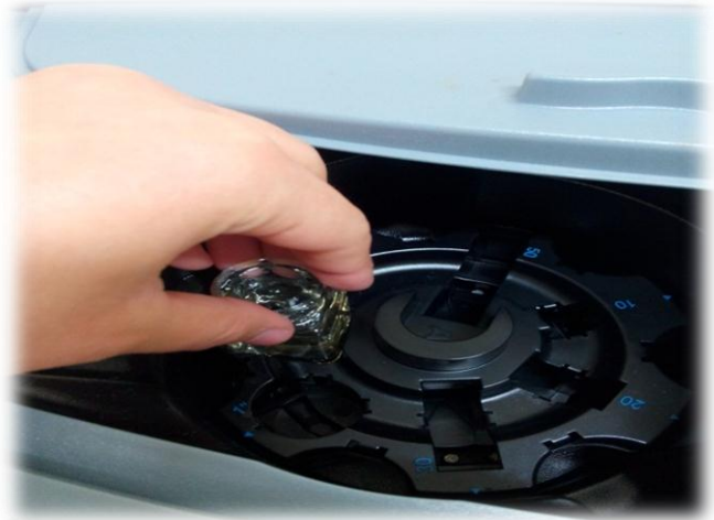
Figure 6.13: the cuvettes were put in the spectrophotometer to be tested
