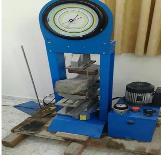
Figure (3.10): Set up of flexural tensile test .
