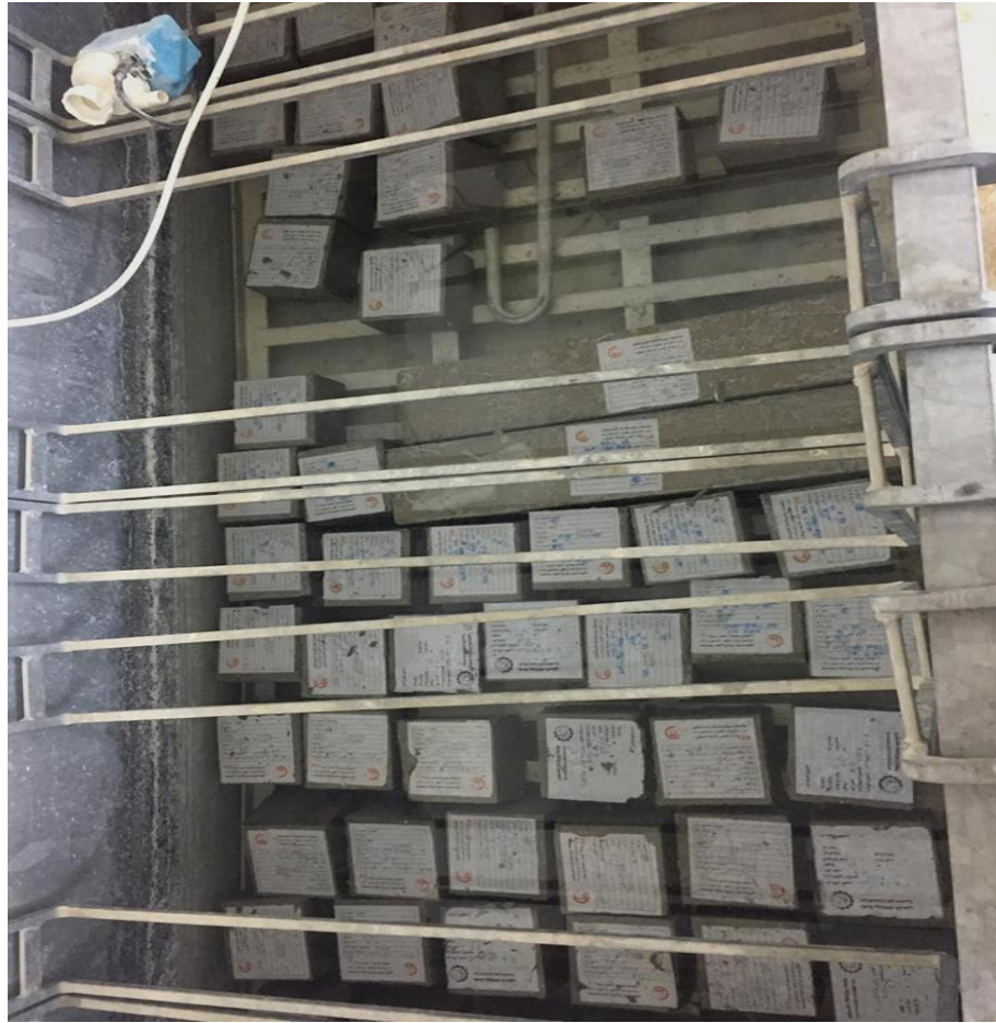
Figure (3.5): Concrete in curing stage.
