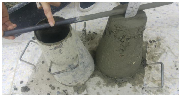
Figure (3.7): The slump measurement
