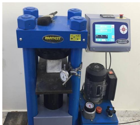
Figure (3.9): Set up of compressive test .
