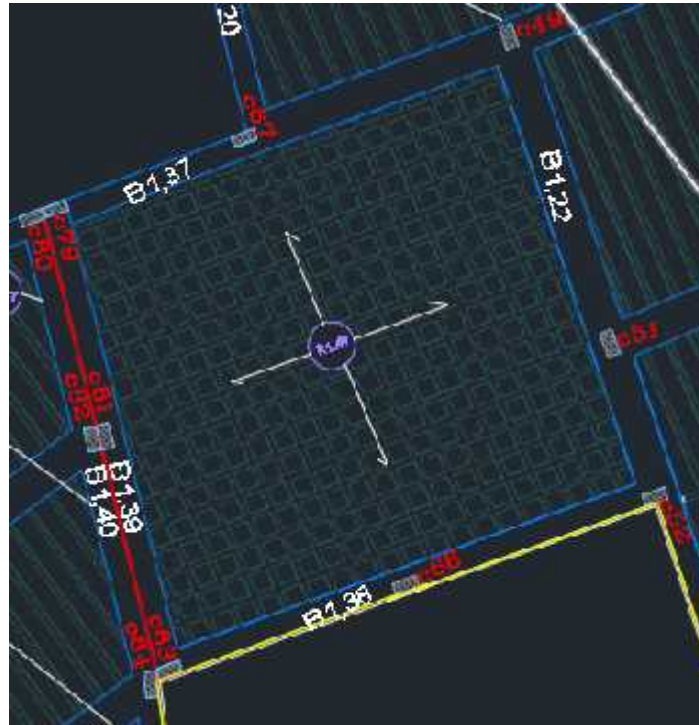
Fig 4.8: Tow Way Rib Slab
