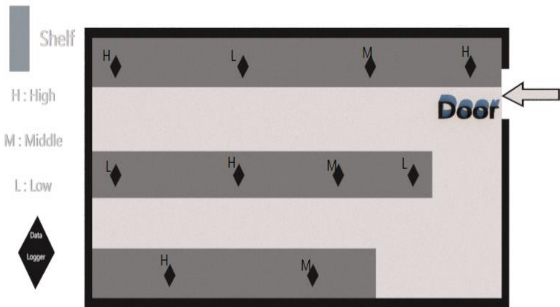
Figure (4.2) Locations of sensors
