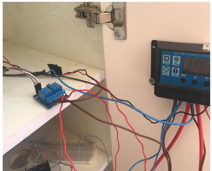
Figures 5.5: Battery connected with relay module and charger controller
