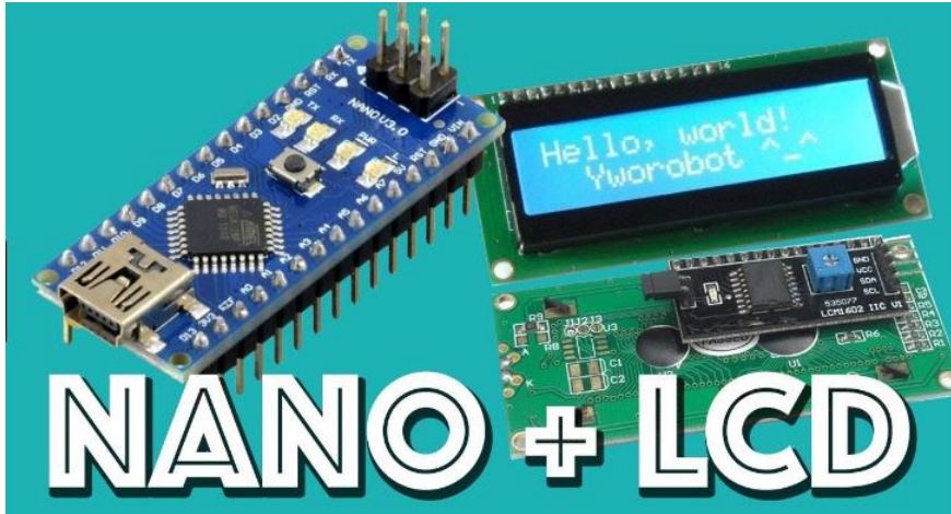
Figure 4.15 Nano Arduino and LCD screen
