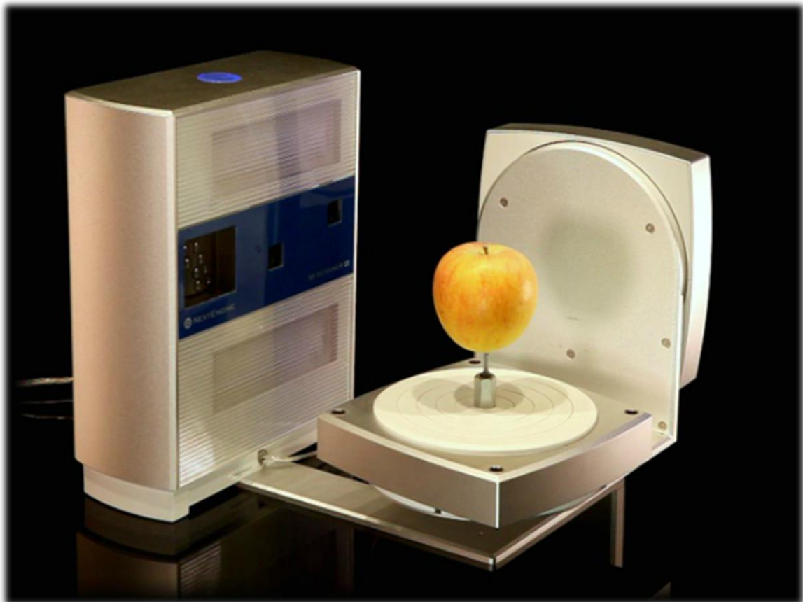
Figure 3.6: Multi Stripe Laser Triangulation (MLT)
