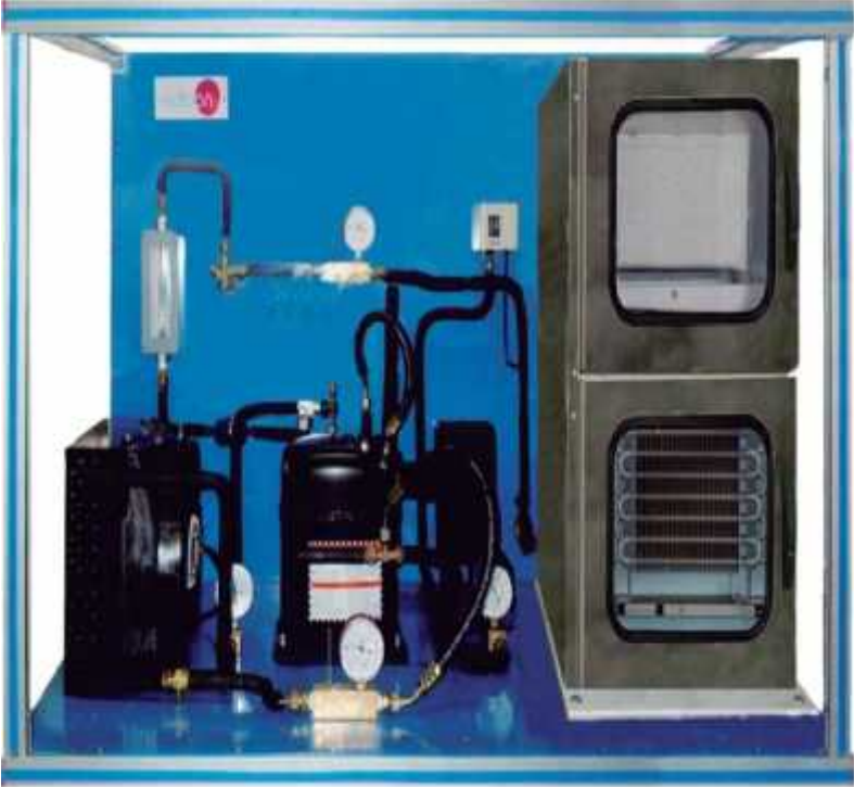
Figure 2.4:Refrigeration unit with refrigeration and freezing chamber
