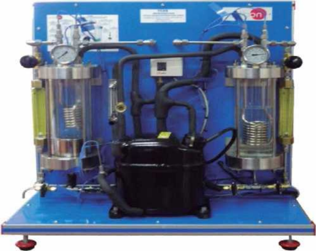
Figure 2.3:Refrigeration cycle demonstration unit
