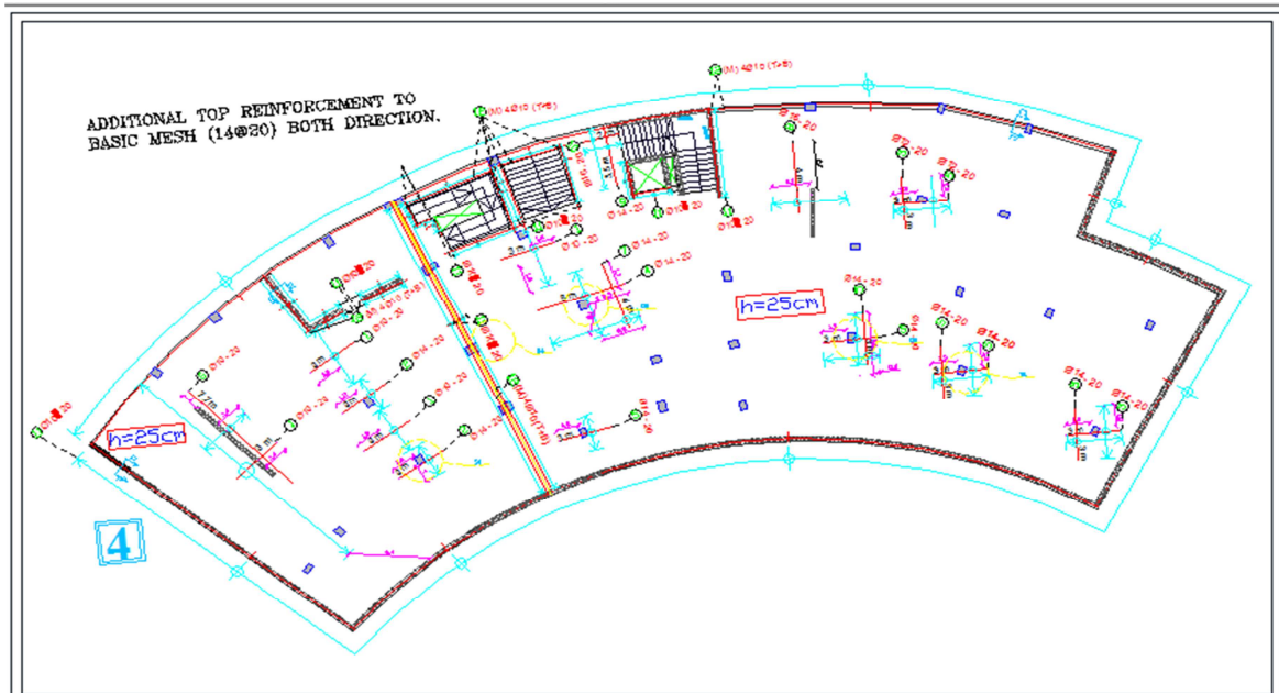
Fig. (4- 31 ) : Top flexural steel reinforcement .
