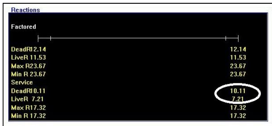
Fig. (4-15) : Span1 service load from rib103.
