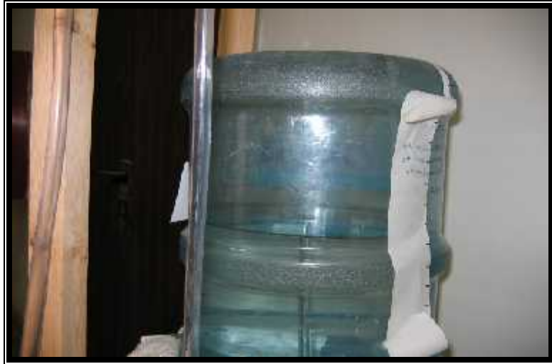
Figure A-22: Gas meter device
