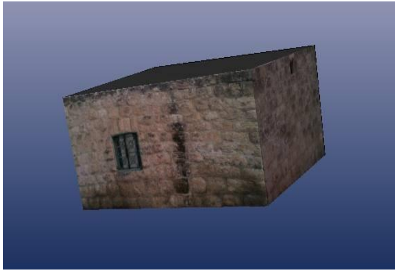
Figure(5.9) 3D model of the house by a variable distance from the house by Photomodeler software.
