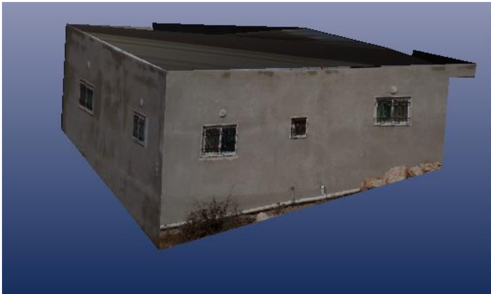
Figure(5.2) 3D model of the house by fixed distance 10 m from the house by Photomodeler software.
