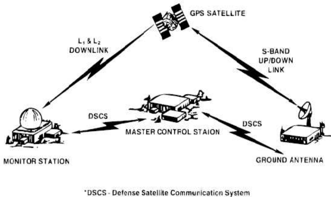
Figure 2.4: Monitor Station and Ground Antenna 1
