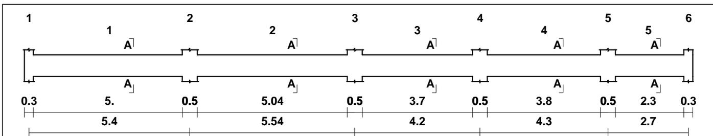
Figure (4-6) : Beam Geometry.
