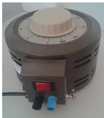
Figure 3.5: 0/260 V I phase autotransformer.
