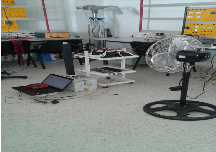
Figure 5.7: Using change speed fan in experiment.
