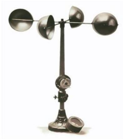
Figure3.13: Anemometer used for measuring wind speed.
