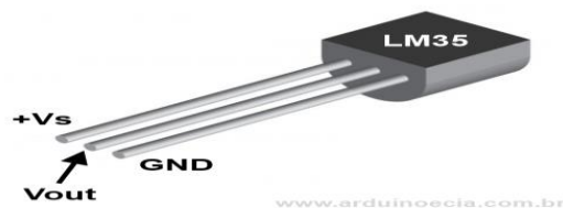
Figure3.9: The temperature sensor that used in experiments.
