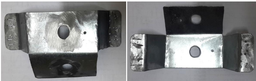
Figure 5.14: Front and Ground sensor metal holder.
