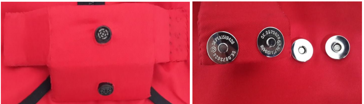
Figure 5.16: Front and Ground sensor metal holder covered by red fabric.
