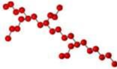
Figure 2.2: A polymer molecule with branching. [6]
