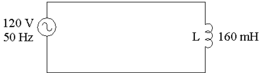
Figure 2-7 simple AC circuit with purely reactive load
