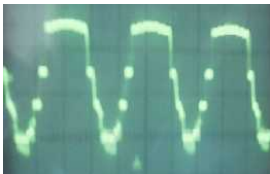
Figure-6.10(Phase waveform when using the capacitors)
