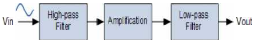
Figure (3.11):- Active Band Pass Filters Construction.
