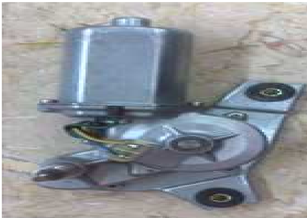
Figure (3.19):- Power Window Motor LH.[22]
