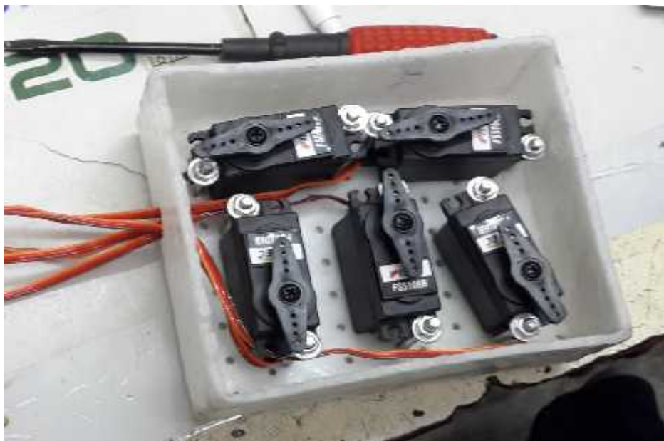
Figure (5.3):- FixedThe Five Servo Motor in Box That Made of Polyethylene.
