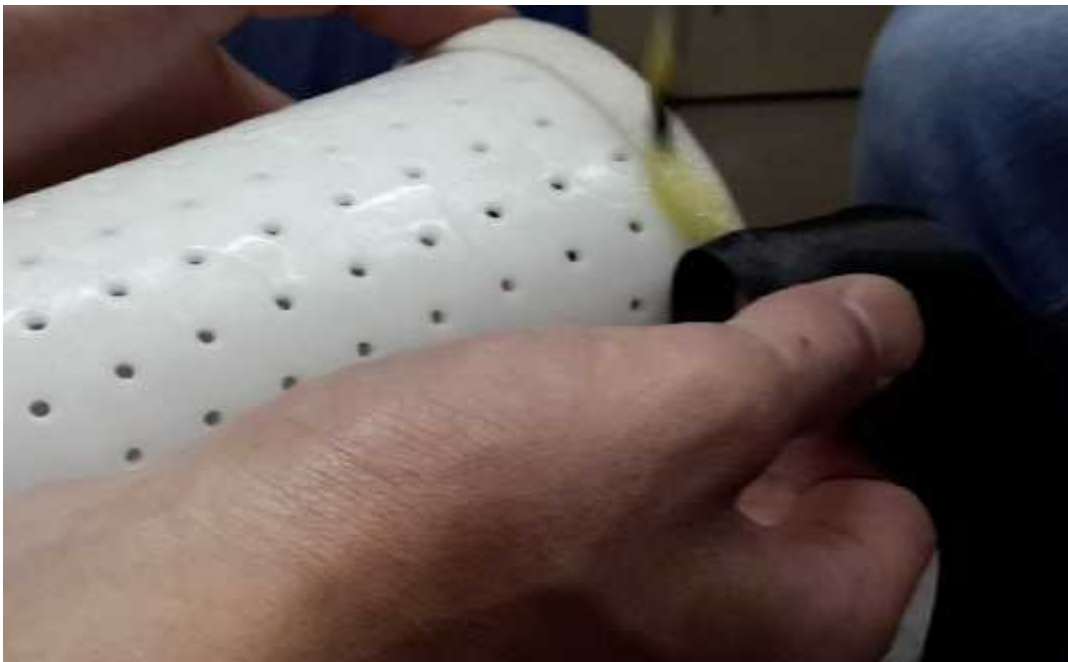
Figure (5.1):- Forming Artificial Arm Using Polyethylene.
