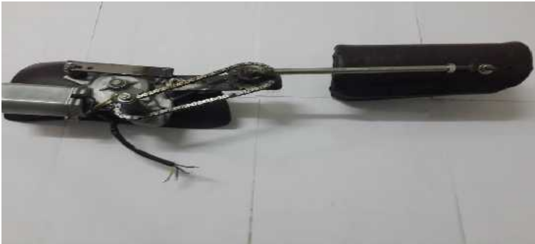
Figure (5.5):- Mechanical Design of Hand.
