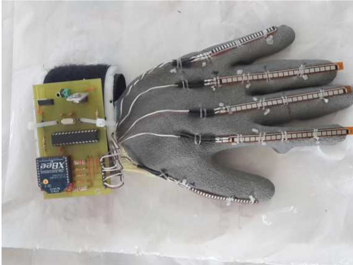
Figure (5.6):- Installed The Flex Sensors on The Fingers
