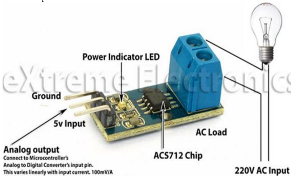
Figure 2.13: ACS712 current sensor components [15].
