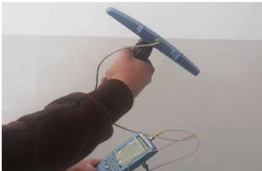
Figure 5.1: The receiving antenna at 900 MHz is adjusted at - 45 degrees
