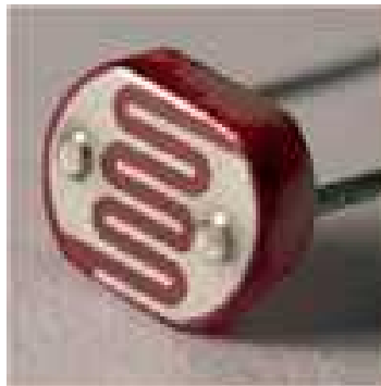
Figure (3.8): The photo resistor (see appendix 3)
