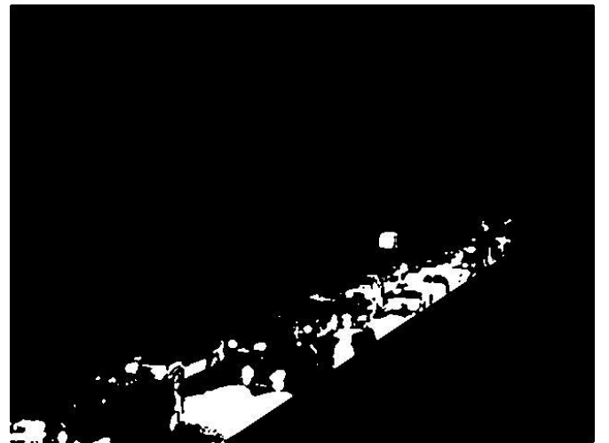
Figures 5.32 and 5.33 Median filtered image, converted to binary image, complemented
