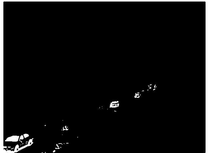
Figures 5.14 and 5.15 Median filtered image, converted to binary image, complemented
