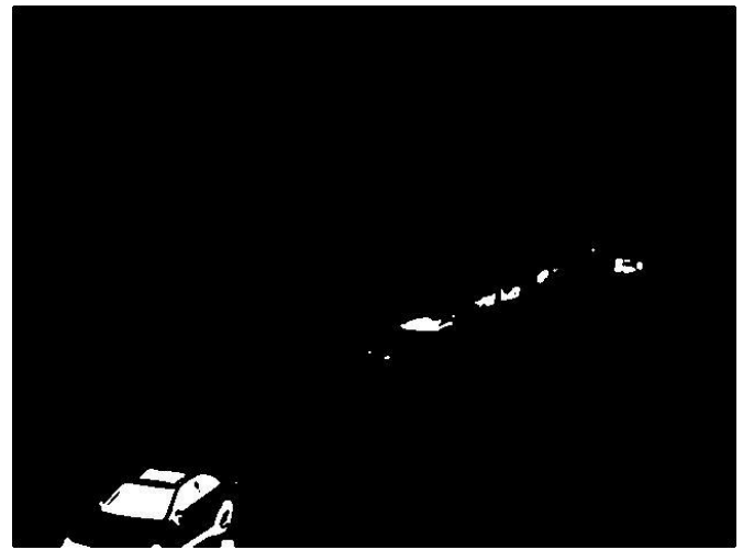
Figures 5.22 and 5.23 Median filtered image, converted to binary image then complemented
