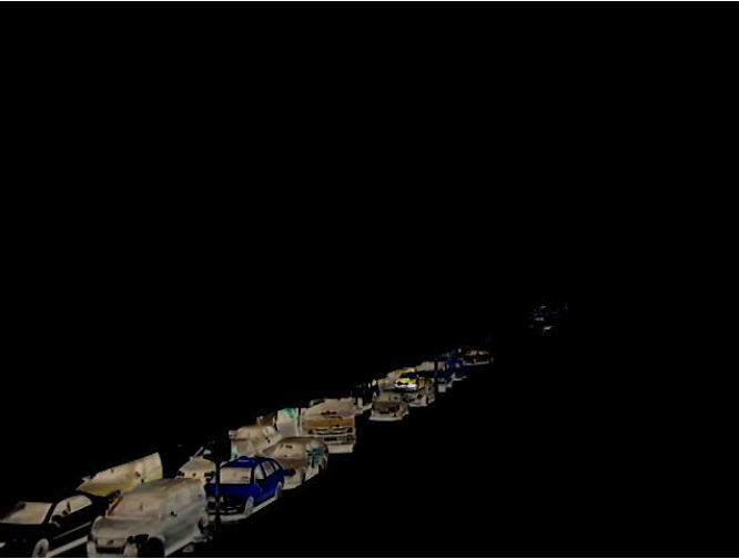
Figures 5.2 and 5.3 Subtracted from the reference image, complemented and brightness-adjusted
