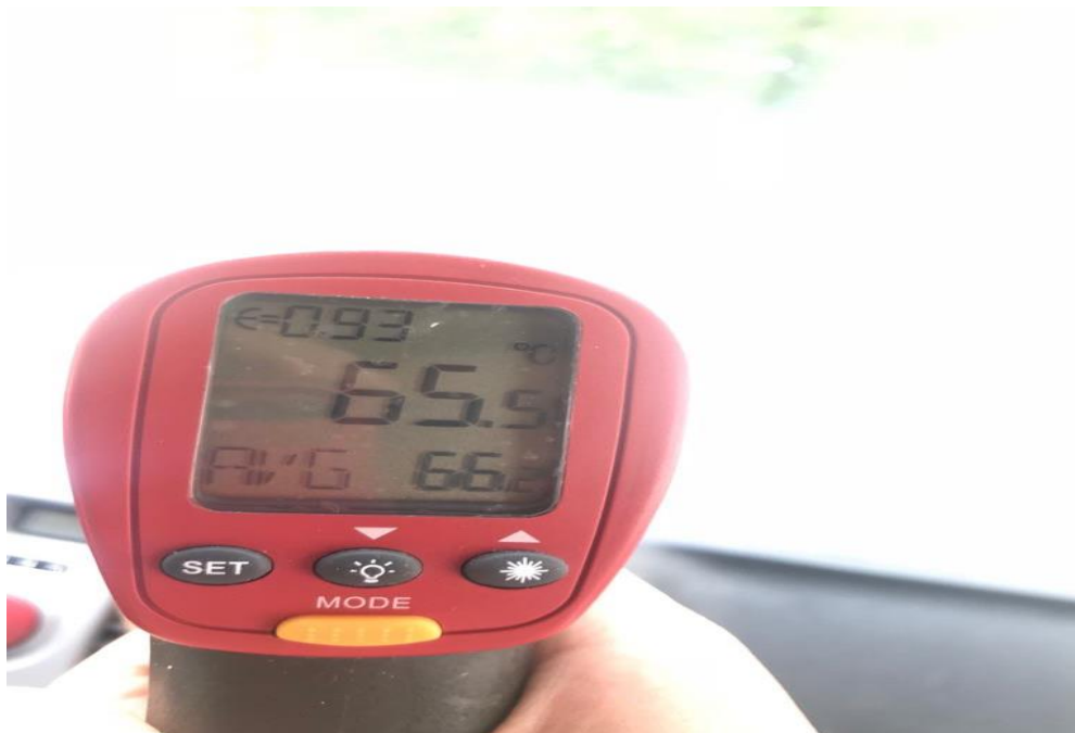
Figure 2.4: Measured Temperature in Vehicle Front position
