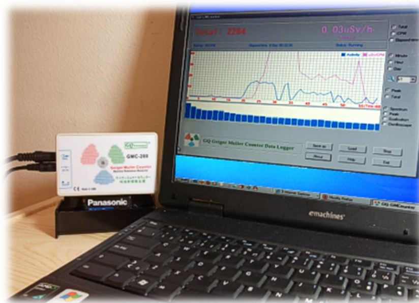
Figure 4.11: Geiger Counter Computer Connection [56]
