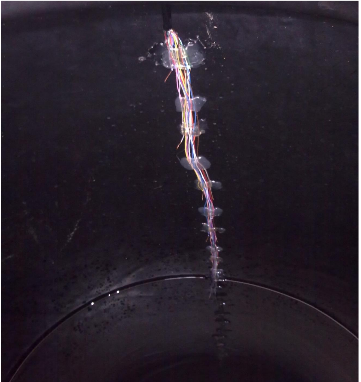
Figure (6.3) The level Sensor in the Main Tank.
