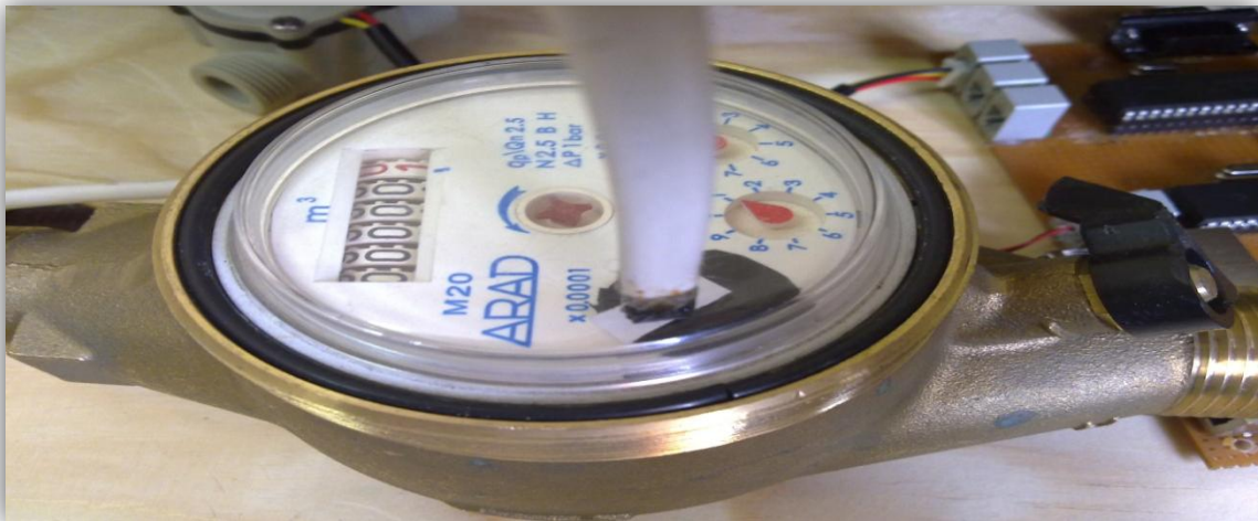
Figure(5.3) Analog flow meter and the transceiver sensor
