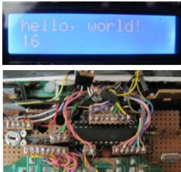
Figure 5.2 : ATmega 328 (#2) microcontroller test circuit.
