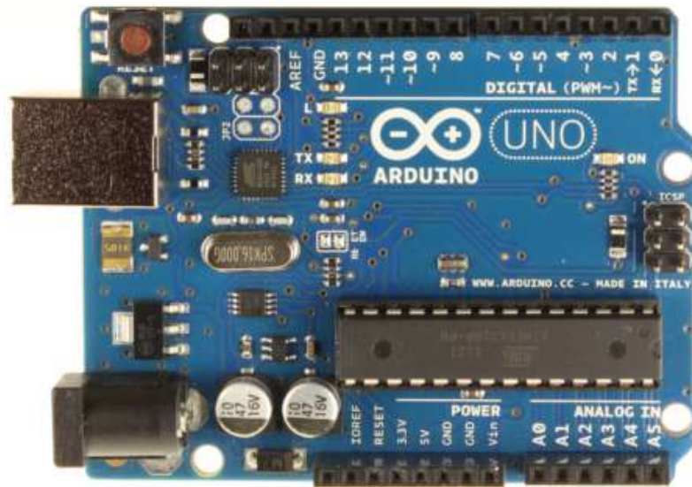
Figure 2.4 : ATmega 328 microcontroller on arduino board.
