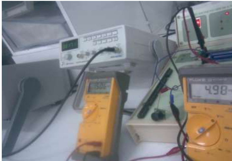
Figure5.9: Output voltage when object located along distance from the sensor. Distance =391.4cm
