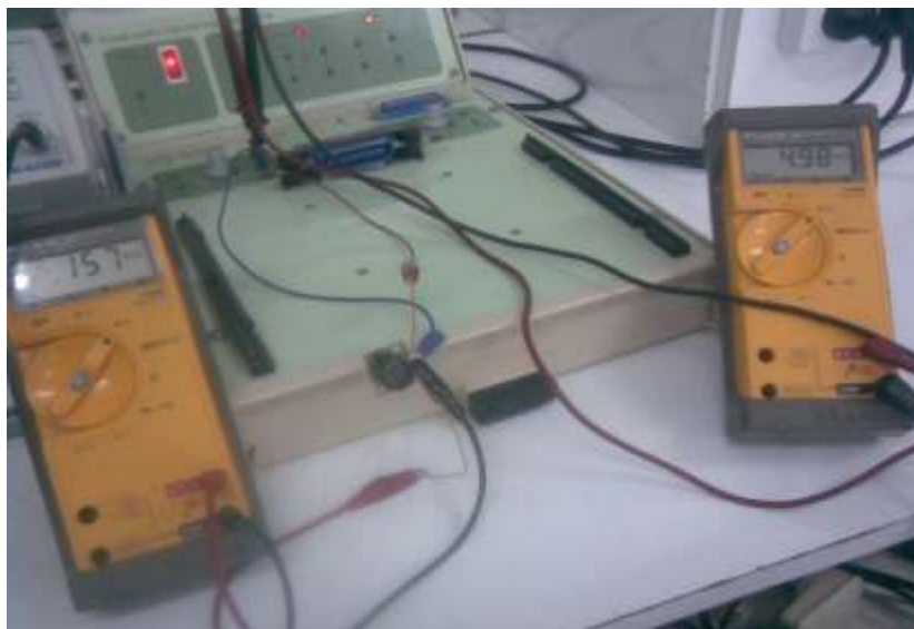
Figure5.8: Output voltage when object located a small distance from the sensor. Distance =40.7cm
