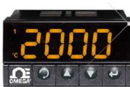
Figure (2.26): Auto-tune PID Controllers
