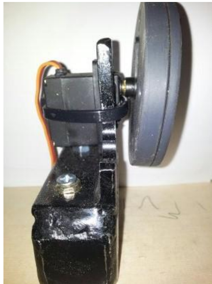
Figure ( 5.5 ): Wheel of filters with servo motor
