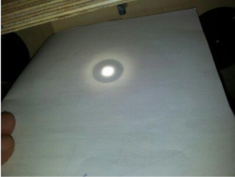
Figure (5.10): Test the Double convex lens and how its concentrate the light.
