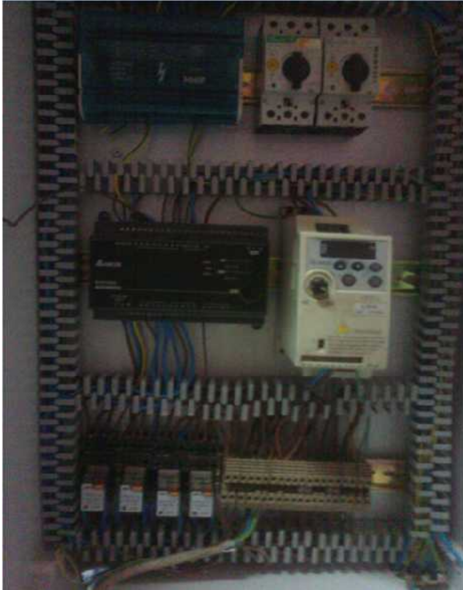
figure 4.9 : layout of control panel of machine
