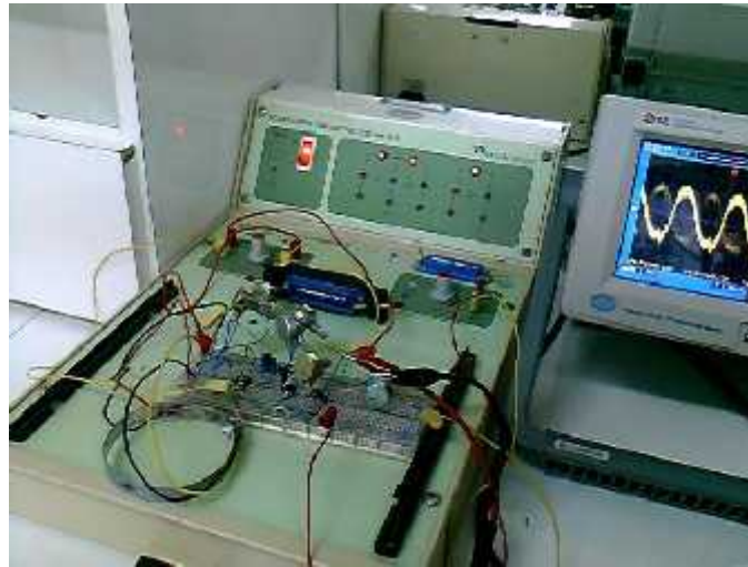
Figure 6.14: Test of the Bridge and Band Pass Filer Circuit
