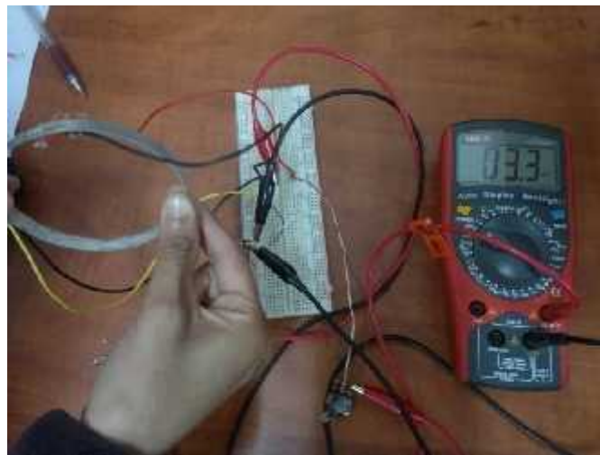
Figure 6.5: the output voltage after pull the ring in two sides
