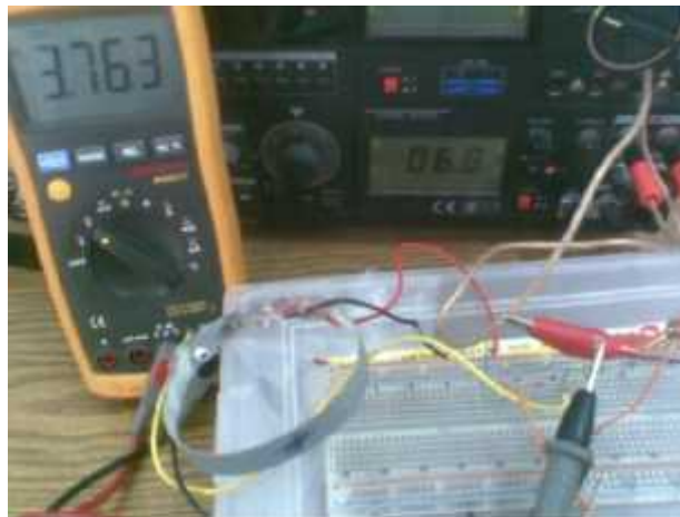
Figure 6.9: The output voltage of the 1k resistance with connection of outer strain gage sensor without making strain
