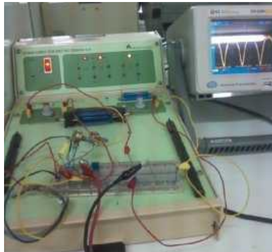
Figure 6.13: Test of the Bridge and Differential Amplifier Circuit
