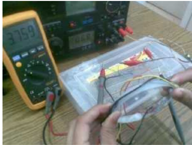
Figure 6.8 :The output voltage of the 1k resistance with connection of Inner strain gage sensor with making strain
