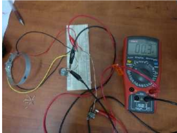
Figure 6.4: the output voltage before pull the ring in two side
