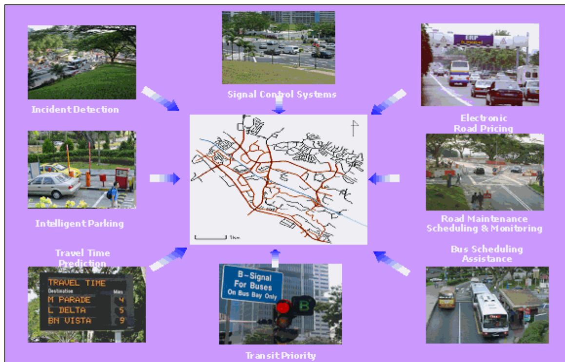
Figure 2.4: Various intelligent transportation systems components.
