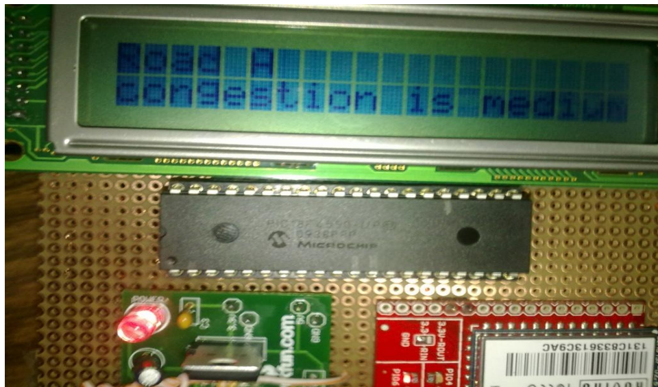
Figure 6.7: Message shown on the LCD when congestion is medium
