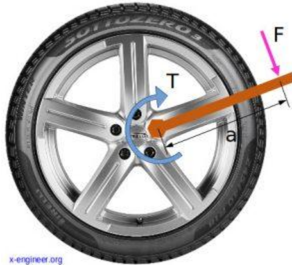
Fig 6.1 Tightening torque at wheel bolt
