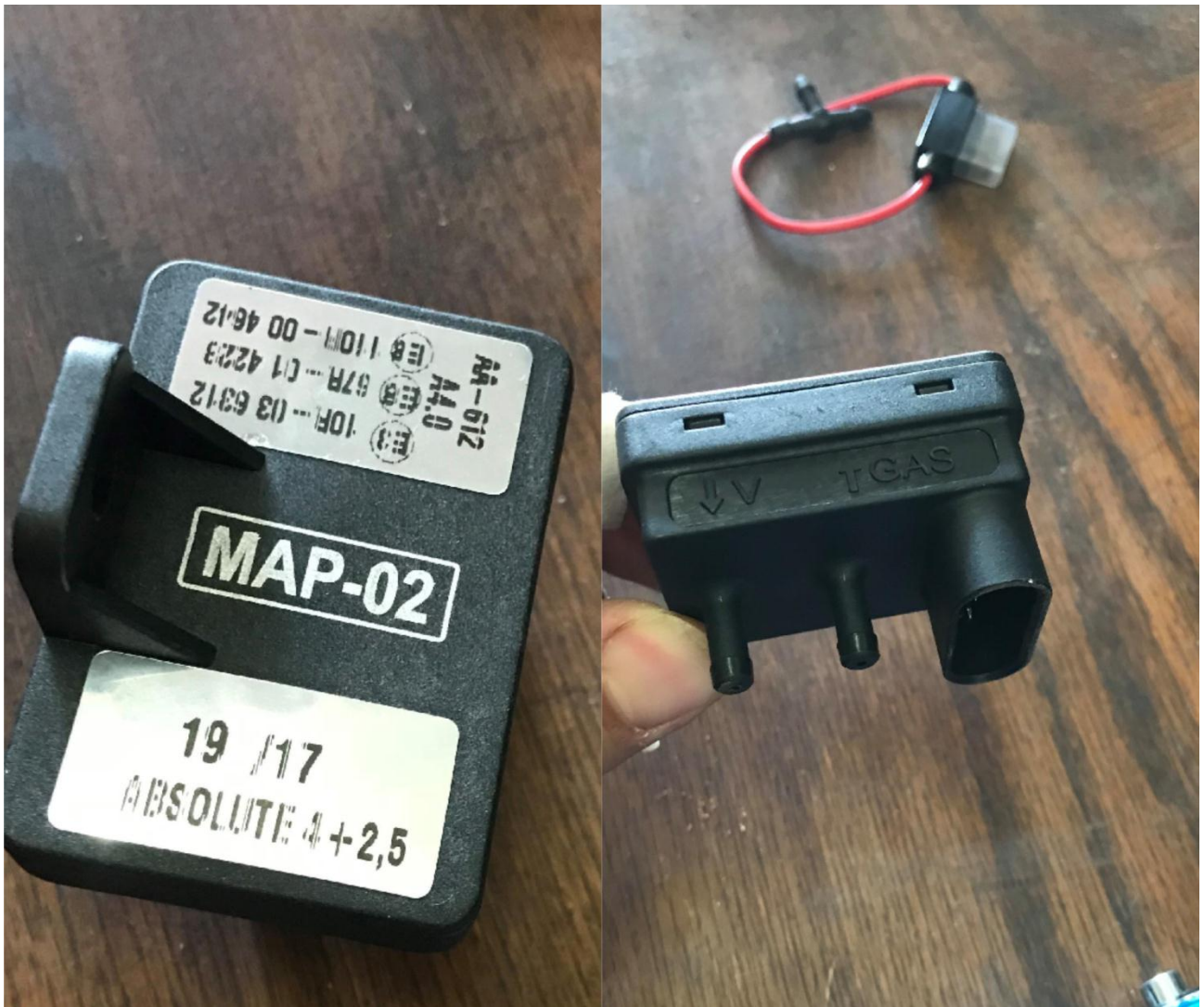
Fig 3.5 Mimigas MAP Sensor.
