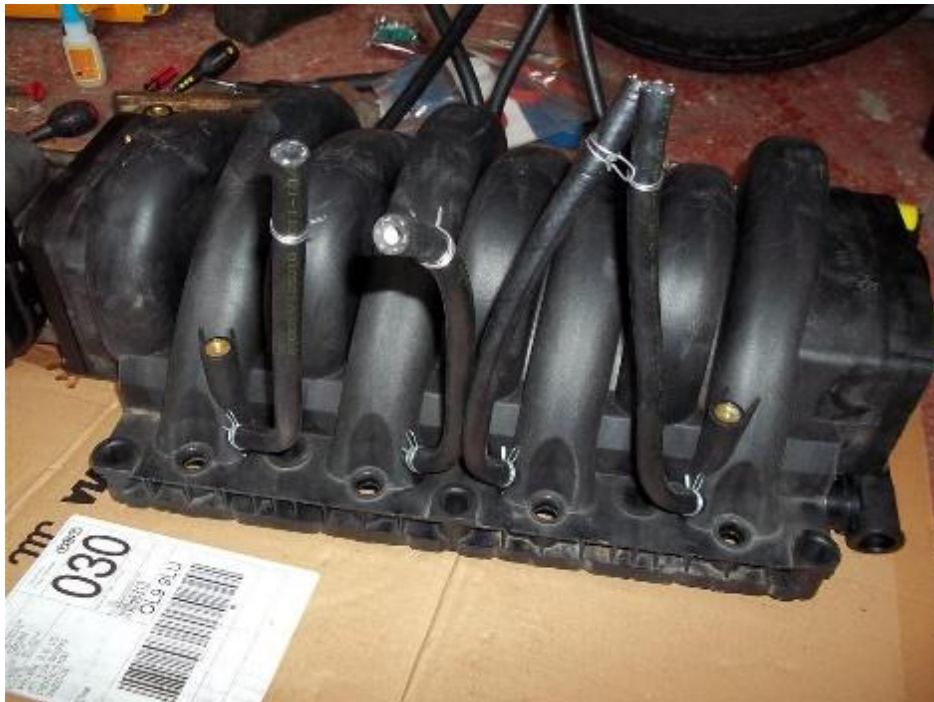
Fig. 5. 1 Fitting of Nozzle for Intake Manifold.
