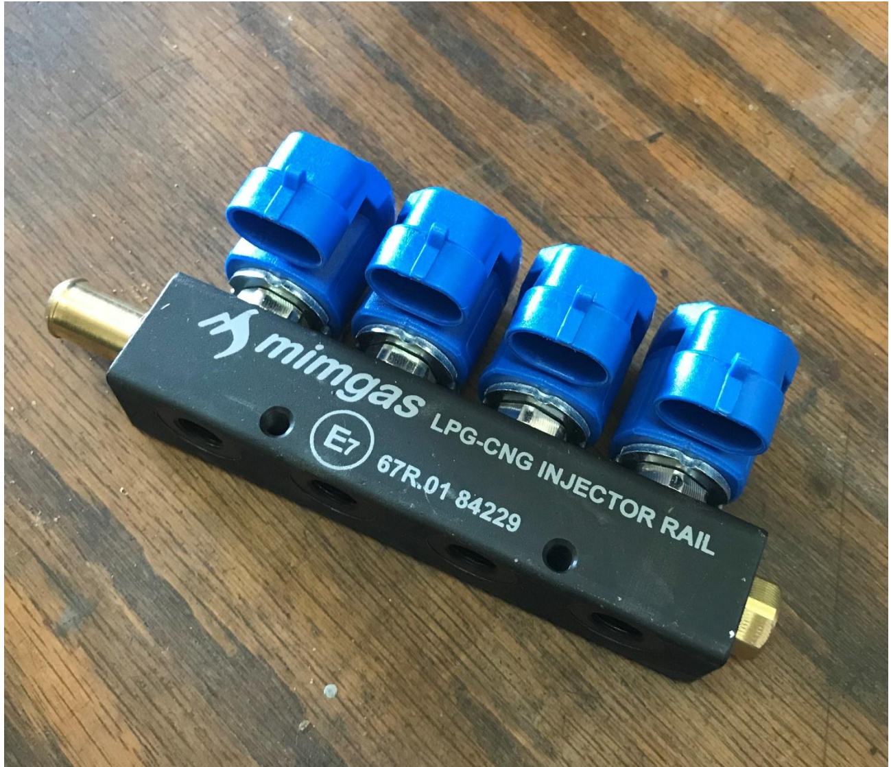
Fig 3.3 Mimgas Injector Rail.
