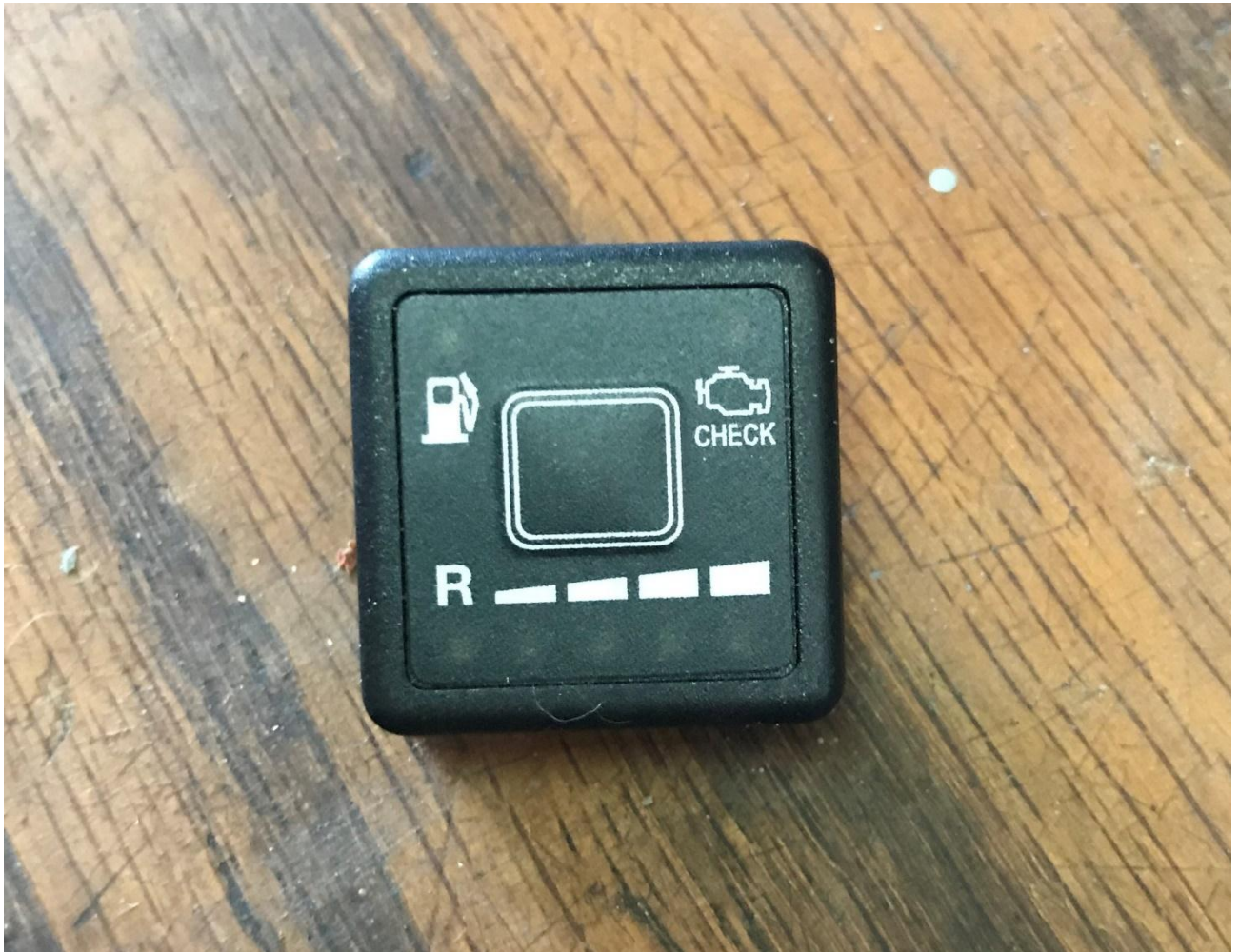
Fig 3.10 Mimgas Changeover Switch.
