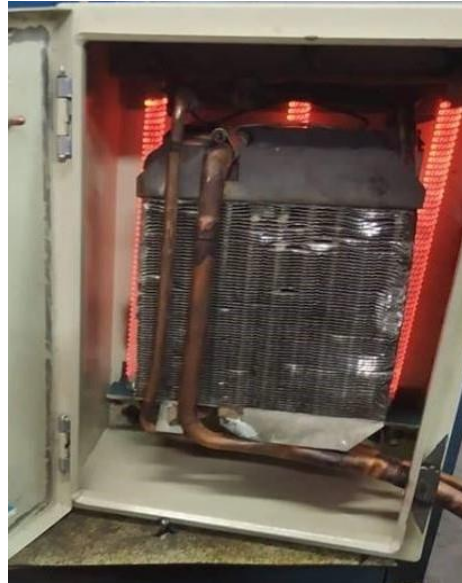
Figure (3.10): Testing the electric heater coils.
