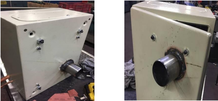
Figure (3. 7): The container after welding the ports.
