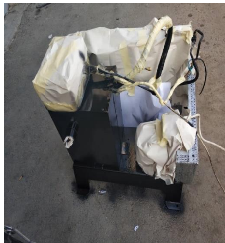
Figure (3. 15): The heating and refrigeration unit after painting.
