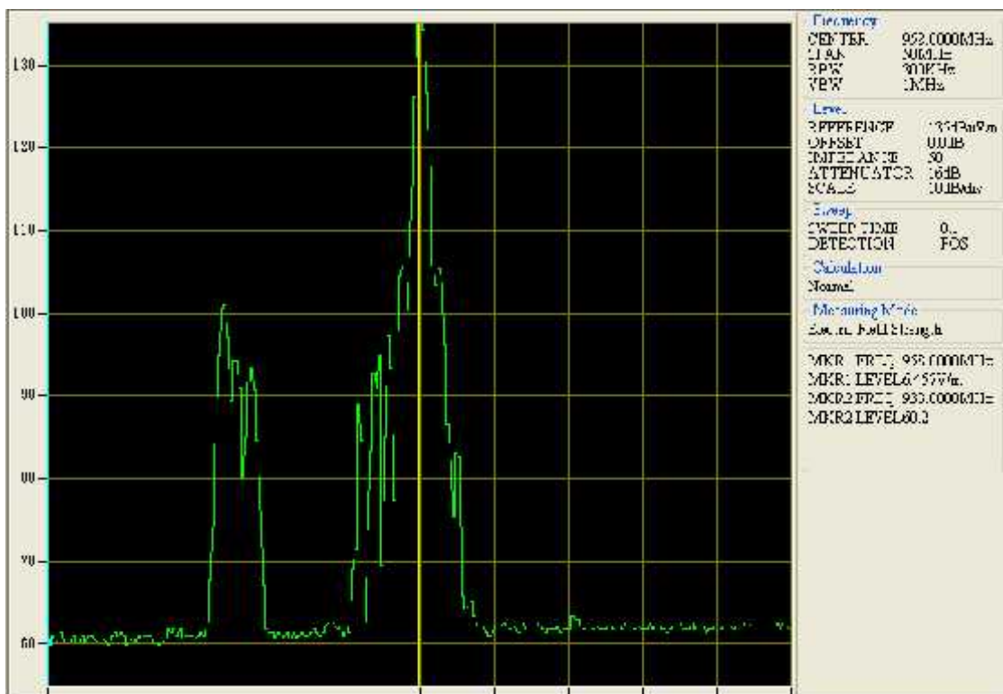
Figure 4.12: Electric field measurements at distance 3m away from Ein Sarah base station (cell C).
